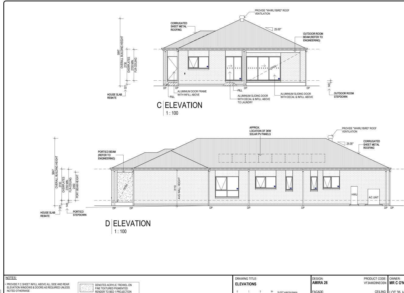
RENDER TO BED 1 PROJECTION THE RENDER PROCESS IS TO BE APPLIED OVER THE CAULKED ARTICULATION JOINTS AS PER METRICON STANDARD PRACTICES.
